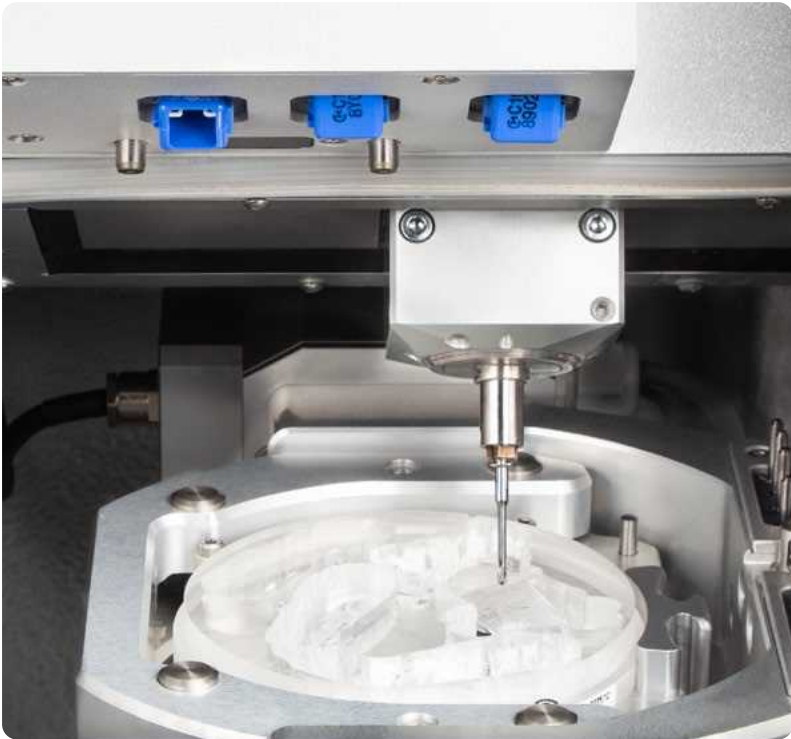
The three integrated ionizers (blue nozzles) neutralize the static charge of acrylic chips – for a clean working chamber and minimal cleaning effort.
