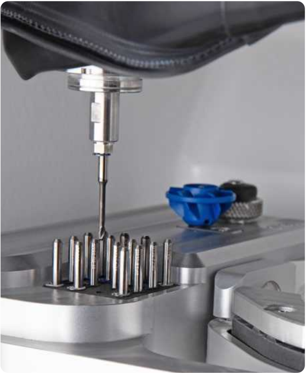
The automatic tool magazine with space for 16 standard tools plus an airtool .
