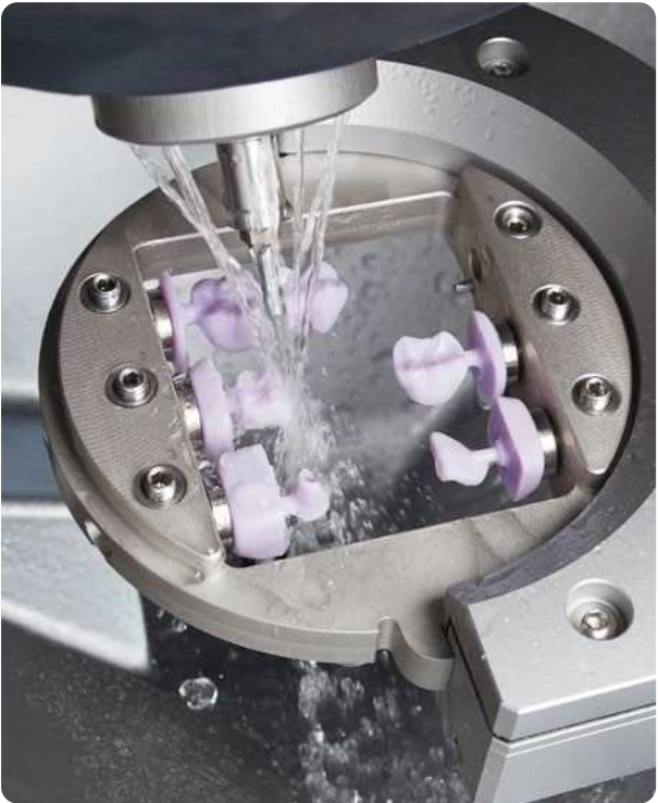
During wet processing, the R5 grinds with clear water – better for your materials and without annoying disposal. And thanks to directclean Technology, even when quickly switching to dry processing.
