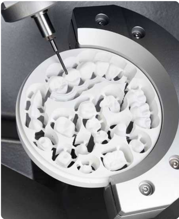
The R5 tilts the spindle (B-axis) by up to \pm 35^\circ . This means that the blank holder only needs one moving axis (A-axis), thereby making the entire system more stable.
